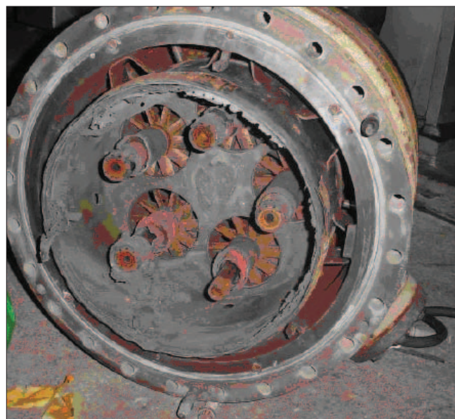
Figure 6.9 – Impact of Combustion Dynamics and Combustion Oscillations.
